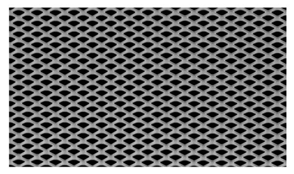
LW Pitch:10.00mmStrand Width:1.75mmSW Pitch:6.50mmThickness:1.20mmWeight:5.08 kg / m2Open Area:46%
